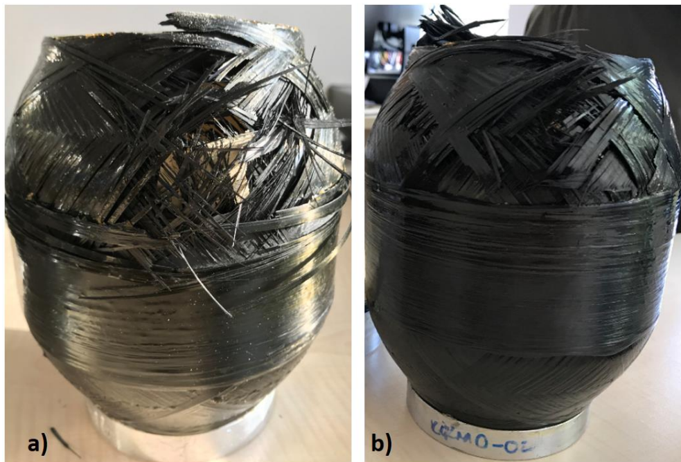
Figure 4.18 Burst modes of the XOXOO windings a) DC b) DLS
