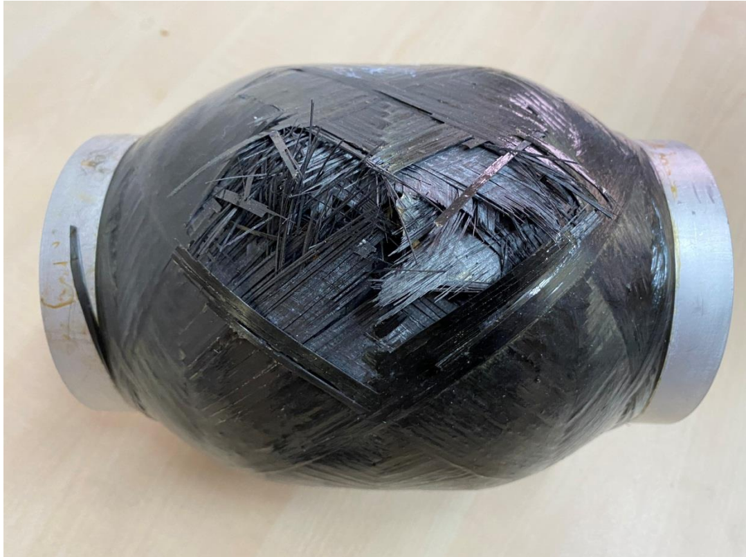
Figure 4.9 Macro image of XOX COPV (with no defect) failure surface.
