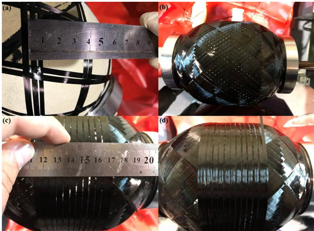
Figure 3.15 (a) 1.0-1.5 mm spaced winding of helical layer in COPV (b) spaced wound helical layer (c) 1.0-1.5 mm spaced winding of hoop layer in COPV (d) completed spaced wound XOX COPV sample
