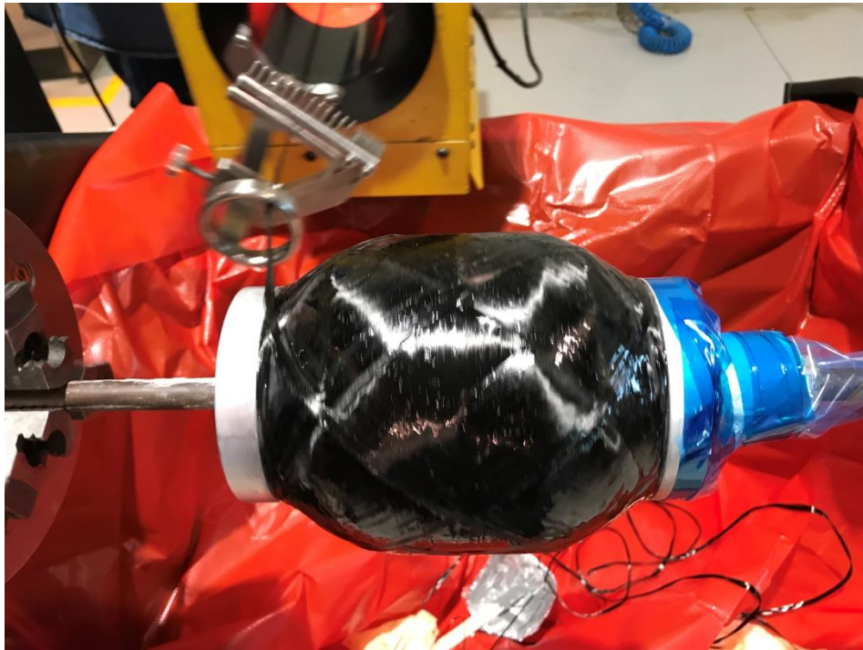
Figure 3.10 Helical layer winding process of XOXOO COPV sample
