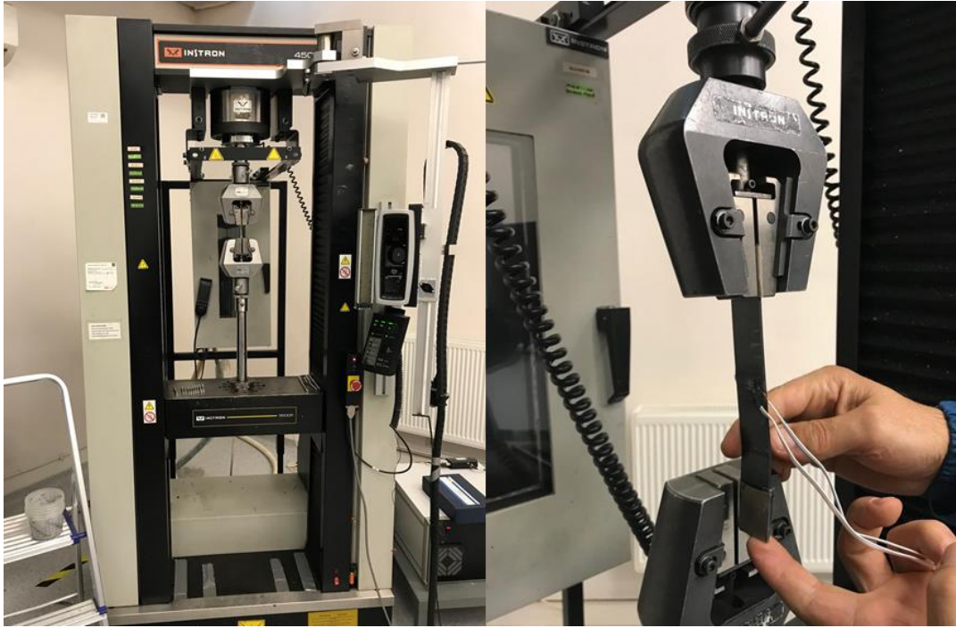
Figure 3.3 Transverse tensile testing setup of carbon/epoxy coupons
