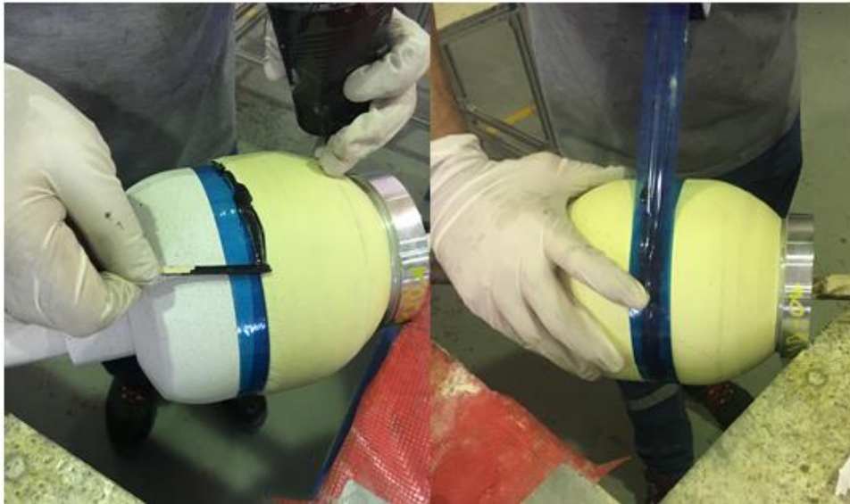
Figure 3.8 Adhesion of EPDM liner on the mandrel
